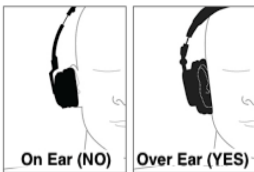
Figure 1: Circumaural headphone with pads covering the ears
