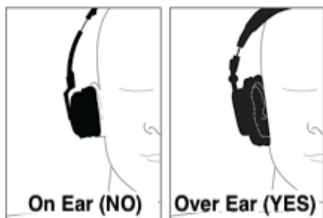
Figure 28: Circumaural headphone with pads covering the ears
